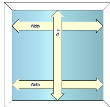
**SUGGESTION:** Some windows may be out of square. 3mm can be deducted from your tight measurements to allow some wriggle room. This is not necessary, but the gaps will be covered by the frame flanges.
