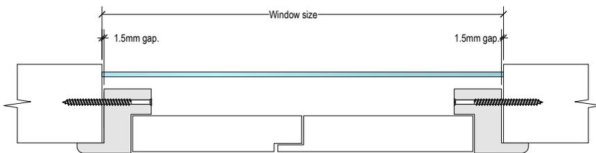
Inside /reveal fitted shutters are mounted inside the window opening with the frame wrapping the edges of the opening.
