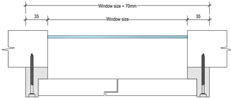
In order to have the frame of your shutters mounted on the window fascia, measure the window opening and **add on 70mm to both the width and the drop.**
